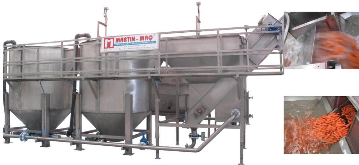
Our innovative SRC series circular soaking system is ideal for prewashing when the raw material (carrots, potatoes, etc.) is very dirty and washing machines have difficulty removing dirt.
