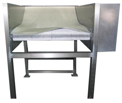
The MC series brushing tables are composed of a series of axes with brushes and are specially designed to brush potatoes, onions, etc.
