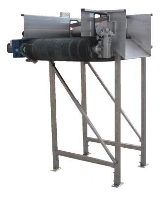
Our range of clod and leaf removers of MEHT series are the right systems to eliminate loose soil and leaves that come with the product from the field.
