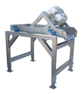
Our range clod removers of VET series are suitable systems to eliminate by vibration clod, coil, dirt and small stones coming from the field.
