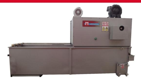
Our range of washing machines by immersion with water, air and final drying of the LIAS series are the perfect machines to carry out a thorough washing of the entire product, including the inside of the leaves and the root, taking advantage of the effect that air bubbles make in its upward movement in the hopper.
