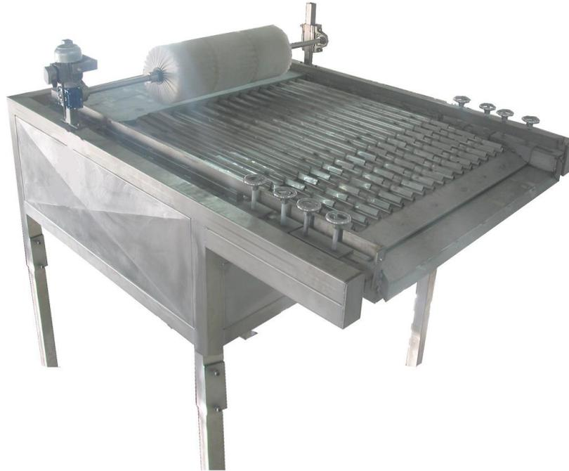
Our range of CALONG vibration length sizers are the suitable systems for longitudinal calibrating, as well as for removing small pieces or aligning the product correctly at the entrance of another machine.
