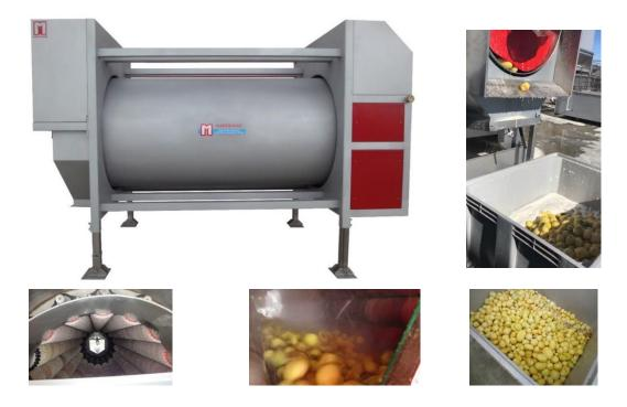
The new range of high-performance, low-maintenance PE series peelers feature a rotating drum made up of rows of peeling brushes exclusively designed by Martin Maq.
