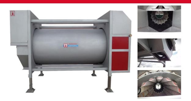
The new PBC series polisher has a rotating drum consisting of rows of brushes exclusively designed by Martin Maq.
