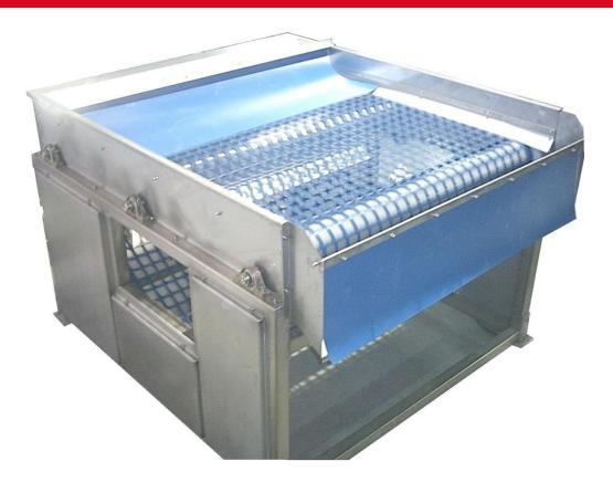
Our range of small piece remover QUIMA series are suitable systems to eliminate small pieces and very small or broken products.
