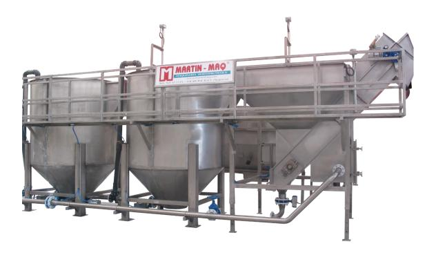
Our unique and innovative SRC series circular soaking system is ideal to perform the pre-wash function when the raw material (carrots, potatoes, etc.) is very dirty and the washing machines have problems removing dirt.
